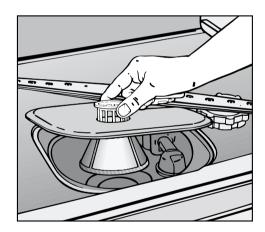
■ Lift the combination filter out of the machine. Remove any coarse particles and rinse under running water. A nylon brush can be used.
